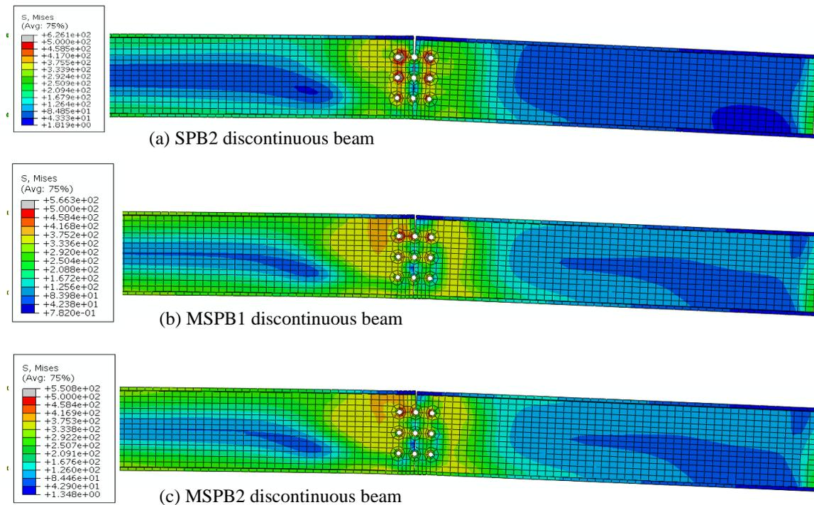
Figure 11. Stress generated on beam due to the conventional and modified SPB connections
