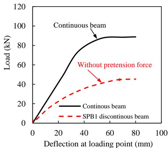
**Figure 7.** Load vs displacement curves of continuous and SPB1 discontinuous beam
