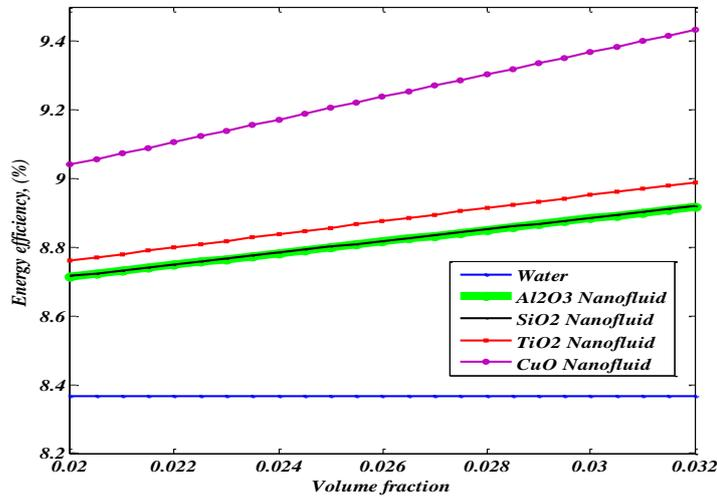
Figure 4. Effect of volume fraction on energy efficiency
