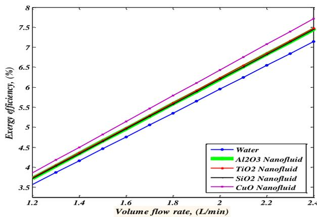
Figure 5. Effect of volume flow rate on exergy efficiency
