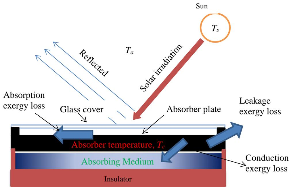
**Figure 1.** Schematic diagram for different exergy losses
