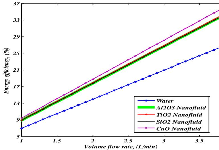
Figure 2. Effect of volume flow rate on energy efficiency
